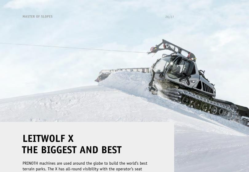
PRINOTH machines are used around the globe to build the world's best terrain parks. The X has all-round visibility with the operator's seat centered and the integrated rear-view camera giving a view of every angle. The increased range of movement of the blade and tiller, the custom-designed park blade with side cutters, and the inclinometer enable perfect execution of park features.
